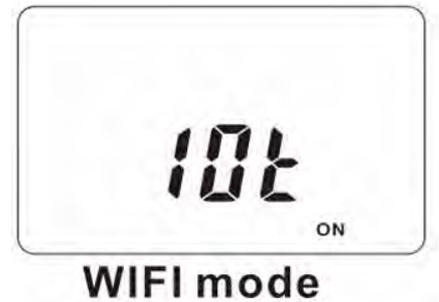
② Press and hold the left key/up key, then press the right key/down key once. Two seconds later, the LCD display will switch from IOT to AP. Then release the left / up key. It has switched to WiFi direct connection mode successfully.
